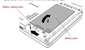
Figure 6-2 Releasing the battery pack (2)
